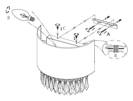
Step 1: Insert masonry plugs into mounting surface A.
