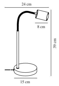
Voltage (V): 230 Volt IP degree: IP20 Maximum bulb wattage (W): 7W Class (Class 1, Class 2, Class 3): Class 2 (Double isolated) Socket type: GU10 Switch placement: On the cable
