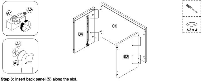
ep 3: insert back panel (5) along the slot.
