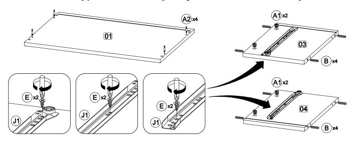
Step 2: Attach side panel (3) and (4) to top panel (1) using hardware A1 and A2 with a screwdriver (not provided).
