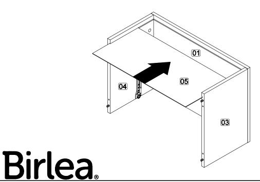
Step 4: Attach bottom panel (2) to side panel (3) and (4) using hardware C and D.
