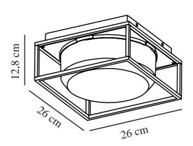
Voltage (V): 220-240 Volt IP degree: IP44
