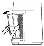
3. Remove the filter from its location 4. Reinstall the filter. and remove the protective film from the filter.
