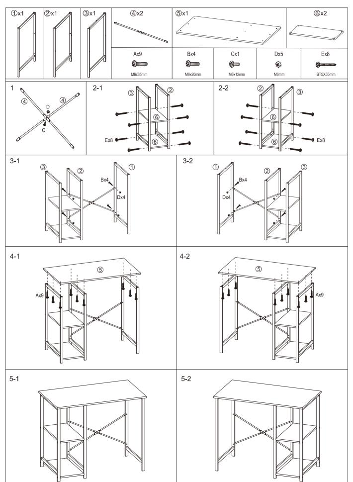
**Notes for installation:** Place **ALL** screws into the appropriate position and then tighten. **DO NOT** place and tighten one by one. If the desk comes with plastic caps, place over screws to cover holes.
