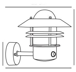
Voltage (V): 230 Volt IP degree: IP54 Maximum bulb wattage (W): 60W Class (Class 1, Class 2, Class 3): Class 1 (Earth contact) Socket type: E27 Parallel connection: True
