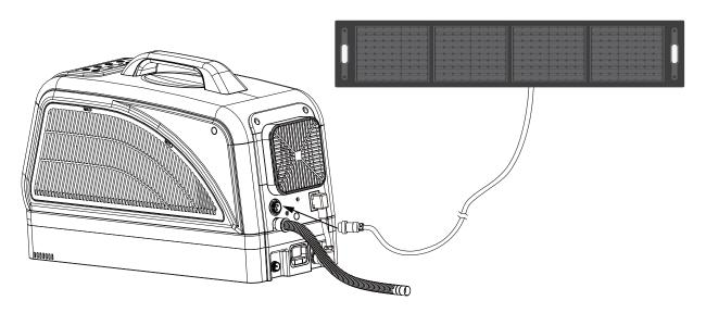
When the air conditioner and the battery are normally connected by the connecting wire, the solar panel can be used to replenish the battery at the same time when the air conditioner is normally started.
