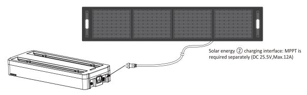
Use solar panels to charge the battery separately
