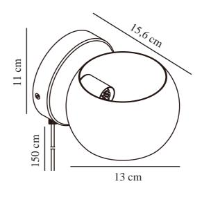
Voltage (V): 220-240 Volt IP degree: IP20
