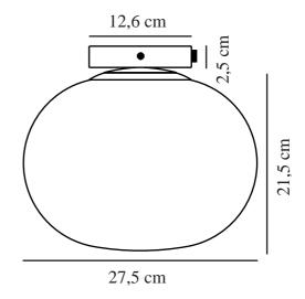
Voltage (V): 220-240 Volt IP degree: IP20 Maximum bulb wattage (W): 25W Class (Class 1, Class 2, Class 3): Class 2 (Double isolated) Socket type: E27
