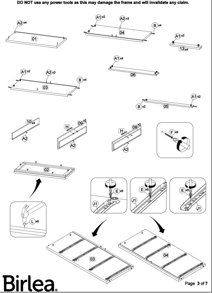
**Step 2:** Attach middle bone (5) and back bone (6) to side panel (3) and (4) using hardware A1 and A2 with a screwdriver (not provided).
