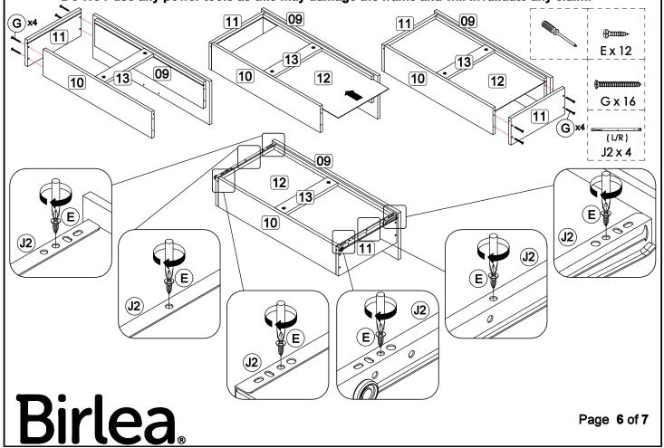
**Step 10:** Assemble the drawer in place along the drawer slides.
