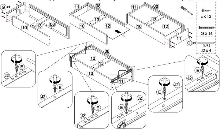
Step 9: Assemble the drawer components using hardware E, G and J2.
