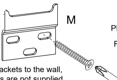
Fix brackets to the wall, screws are not supplied.
