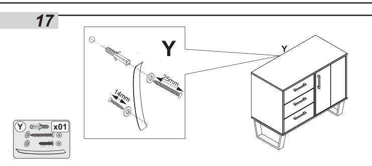
WARNING: CHECK FOR HIDDEN PIPES AND CABLES BEFORE DRILLING.
