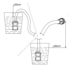
Ensure that the water source is not placed more than 50cm lower than the Pressure Washer inlet.
